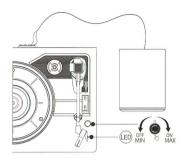
2.After connecting the speaker and plug in the power adapter, turn the power knob (1) clockwise on this unit, Blue indicator light will be on.
